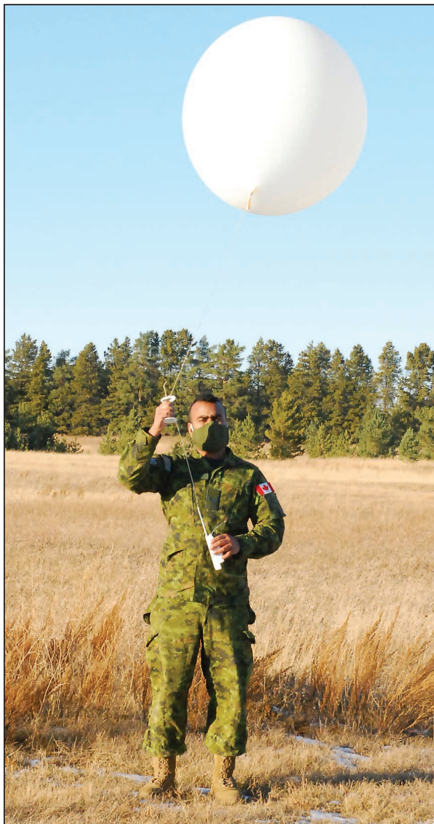
1RCHA Met Tech Cpl Surendran Chandrabose prepares to release a 100gr weather balloon with an attached radiosonde into the atmosphere. Raw data collected from the radiosonde is analyzed by the MW32 sounding system. From here, a METCM message is generated and sent to 1RCHA's Command Post (CP). The crew on the gun line receives target information corrected for atmospheric phenomena from the CP, and firing commences. Photo Kimberley Kielley/Shilo Stag
