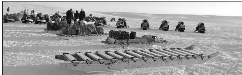
Komatiks are long wooden sleds used by the Canadian Rangers to transport gear behind their snowmobiles. Here, 2PPCLI prepares to go out on a patrol.
