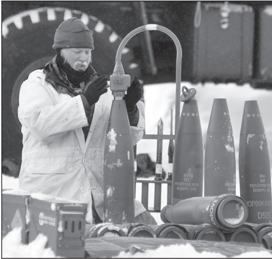
A Precision Guided Kit is added to the M777 shell prior to firing during Ex FROZEN GUNNER.
