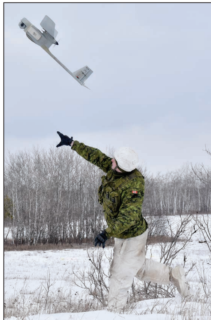
The Raven B is launched into the air by the way of 1RCHA manpower.
