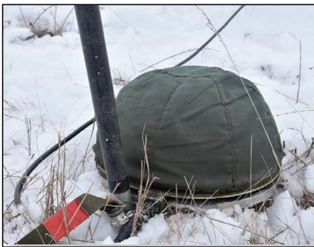
A close up of one microphone from the HALO system used to detect large acoustic events.
