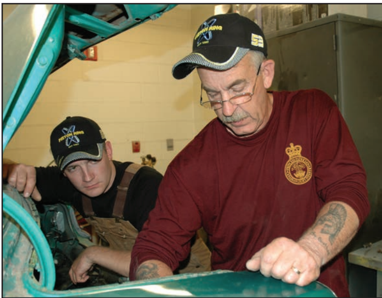
Cpl Mark Ejdrygiewicz, left, looks on as Jim Seggie inspects rivets in the trunk before stripping the vehicle.
