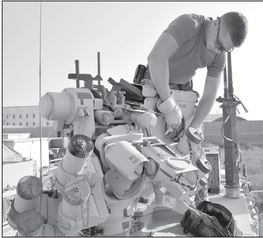
Cpl Kevin Martel, an electronic-optronic technician from 2 Service Battalion, Garrison Petawawa, removes a remote weapons system from an RG-31 Canadian armoured patrol vehicle during Op ATTENTION at Camp Souter, Afghanistan in October 2013.
