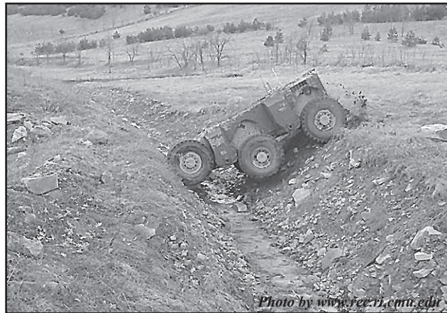
Crusher is able to negotiate difficult terrain such as steep ditches - head on or by angle - even on side slopes of 30°.
