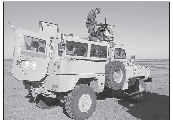
The gunner of an Operational Mentoring Liaison Team (OMLT) loads a C6 7.62mm machine-gun mounted on a Remote Weapon Station (RWS) while conducting live-fire ranges in Shilo. The RWS gives the gunner of the RG-31 Armoured Patrol Vehicle the capability to deliver extremely accurate fire on any target within range.
