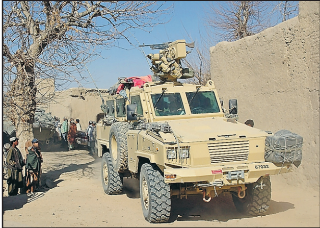
An RG-31 leads a mounted patrol into the village of Sperwan Ghar, south west of Kandahar City. The large windows give the crew good visibility and the C6 mounted on the Remote Weapon Station provides good protection.
