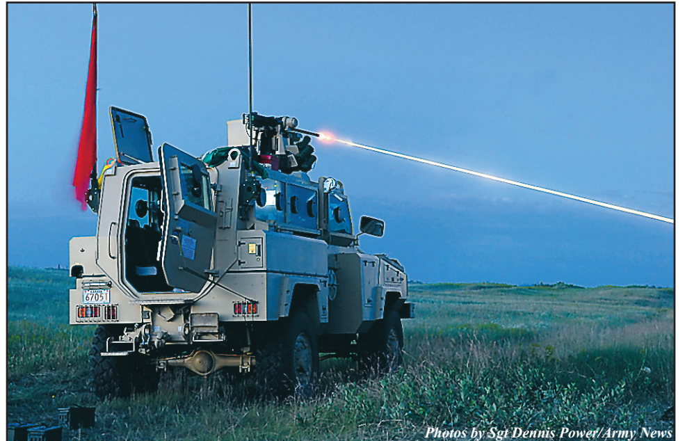
Machine-gunnery engage targets at dusk using thermal imaging sights on the Remote Weapon Station mounted on an RG31. The machine-gunnery are members of 2 PPCLI completing training just prior to a deployment to Afghanistan. The streak of light is caused by tracer rounds.
